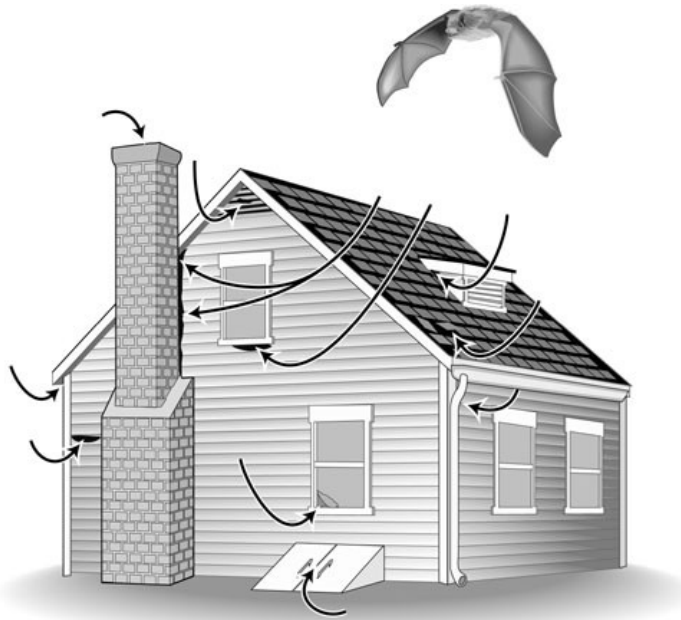
Common entry points on homes and buildings include corners, eaves and louvers.
